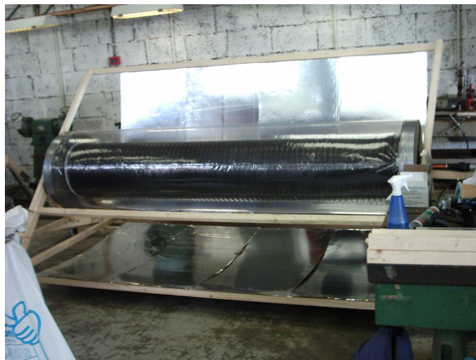
Figure 4.3: Rotating boiler with inflated absorber and cover
