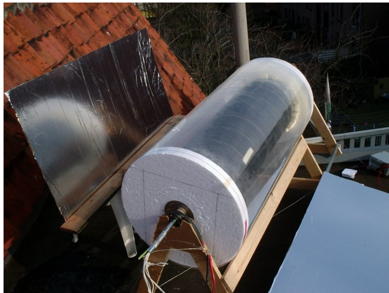
Figure 3.6: Reflectors increase the power input of the collector
