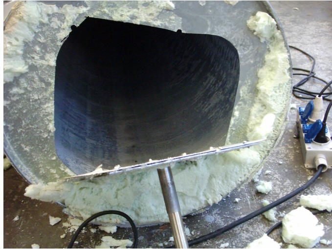
Figure 3.10: Scaling inside the absorber tube.
