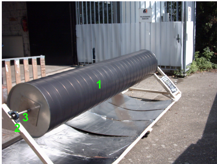
Figure 2.1: Absorber in its frame
