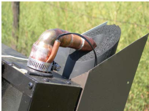
Figure 8. Above, the top-right corner of collector 4, showing the soldered copper piping, some insulation, a thermistor, and a piece of the square-U sheet metal attached to and facing out from the back of the collector. (This photo was taken before I added the air-release vent to this location.) Right, the mating piece of square-U sheet metal has been added. Folds and overlaps between the pieces of square-U shed rainfall from above and from the prevailing wind direction. Below, the transitions from sheet metal covers to underground PVC covers between collectors 2 and 3. (The yellow wire is the unluckily located TV cable.)
