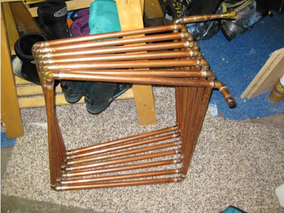
Copper part of heat exchanger
