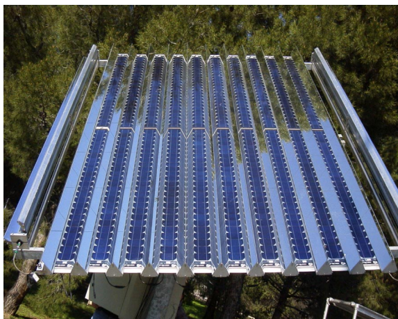
Fig. 2: Frontal view of the ARCHIMEDES concentrator tracking system.
