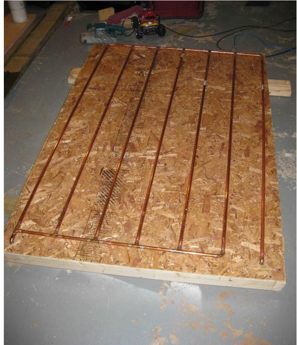
*Illustration 5: This shows the layout of the tubes on the left collector. The top is on the right side of the photo.*
