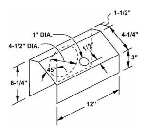
Pop-rivet the fan to the fan shroud, then apply silicone around the edges.
