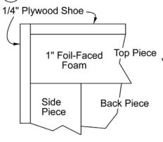
\*Thermax, Tuff-R, Celotex, R-Max, etc, foil-faced urethane (polyisocyanurate) foam
