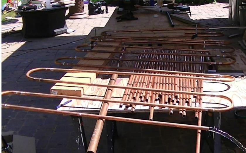
**Leak Testing Pic:** It's best to examine every solder joint very carefully especially on a very hot and humid day where condensation can occur. For best results, plug the outlet with a thumb to pressurize the system.
