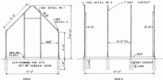
1 NO.14 HEX HEAD SELF TAPPING METAL SCREWS W/ NEOPRENE WASHERS 5 OZ. FIBERGLASS PANELS I" EMT CONDUIT
