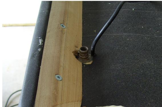
The collector temperature sensor was clamped on the fin close to the pipe at the output end of the collector.
