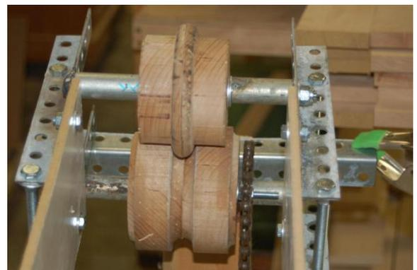
grove. I then bolted a sprocket from the back wheel of a coaster brake bicycle to one of the wheels.
