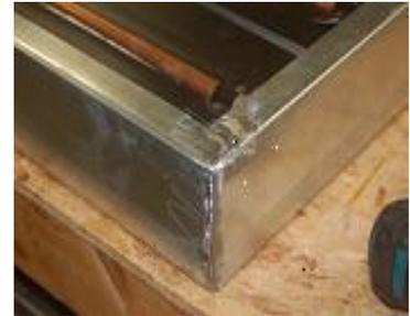
The first panel I made used 20 gauge steel, the other two I used 18 gauge. For the 20 gauge I used sheet metal screws to put it together. The 18 gauge was heavy enough I could weld two corners. After I had two sides and one end put together I was able to put the pipes, insulation and OSB in from the open end, I then installed the other end.
